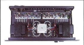
The internal construction of the CAS 1, as in all Threshold products, is unparalleled. An extremely heavy gauge chassis supports the large twin power supplies and thick aluminum "T" beam extrusions upon which the amplifying channels are mounted. All active electronic components are individually selected and tested to insure absolute channel-to-channel and unit-to-unit consistency. Only low noise metal film resistors and tantalum capacitors are used in the signal path.
